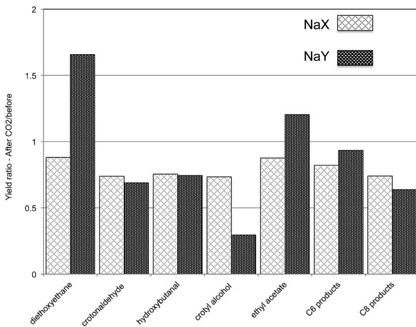
**Fig. 4.** Variation of product yield after exposure of zeolites NaX and NaY to CO<sub>2</sub> as an inhibitor of basic sites expressed as the ratio of individual product yields obtained with and without exposure to CO<sub>2</sub>. Reaction temperature 230 °C, reaction time 6 h, catalyst weight 400 mg, solvent (ethanol)/reactant (acetaldehyde) volume ratio 10, acetaldehyde 2 mL.
