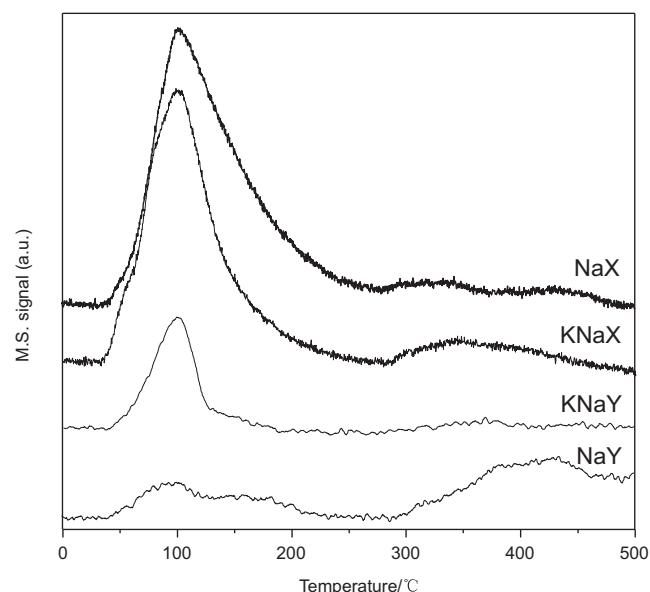
Fig. 1. TPD profiles of CO<sub>2</sub> over zeolite NaX, NaY, KNaX, and KNaY.
