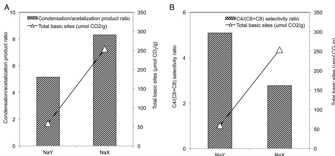
**Fig. 2.** Product distribution from acetaldehyde conversion at 230 °C and 300 psi and basicity of zeolites NaX and NaY.
