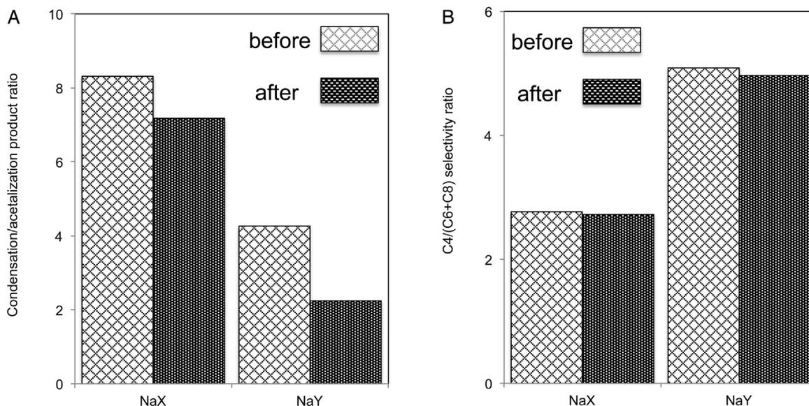
**Fig. 5.** Product ratios over NaX and NaY, before and after exposure to CO<sub>2</sub>. (A) Condensation/acetalization ratio; (B) C<sub>4</sub>/(C<sub>6</sub>+C<sub>8</sub>) condensation product ratio. The solvent (ethanol) to reactant (acetaldehyde) ratio was 10 by volume with acetaldehyde 2 mL. The reaction temperature was 230 °C and reaction time was 6 h. The catalyst weight was 400 mg.
