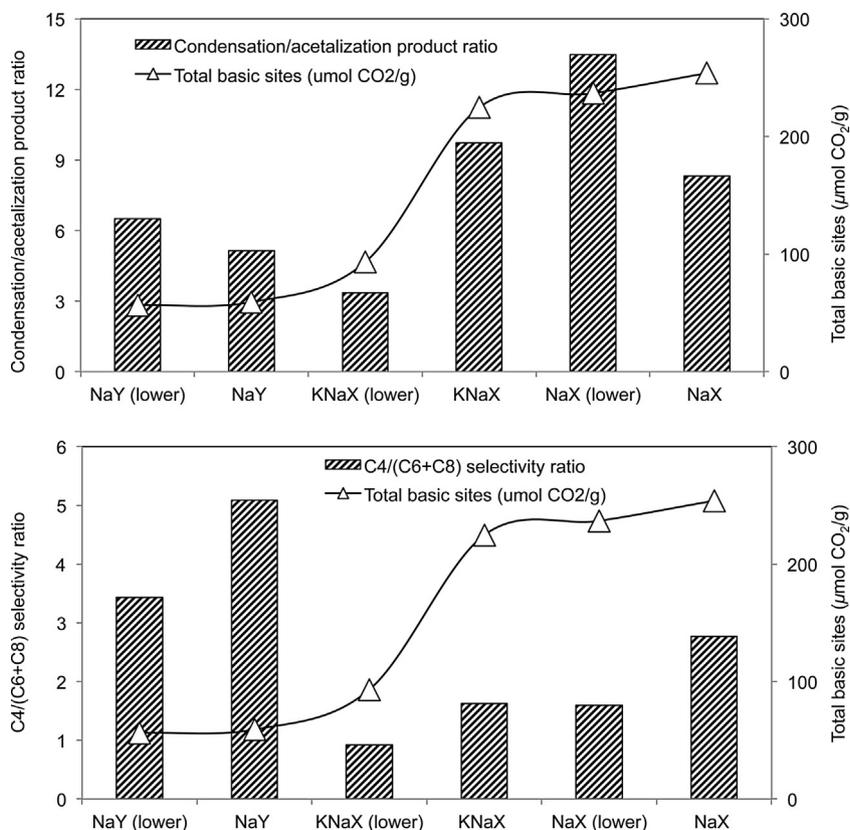
**Fig. 6.** Comparison among zeolites KNaX, NaX, NaY, and the corresponding not fully washed zeolites (lower-water). Reaction temperature 230 °C, reaction time 6 h, catalyst weight 400 mg, solvent (ethanol)/reactant (acetaldehyde) volume ratio 10, acetaldehyde 2 mL.
