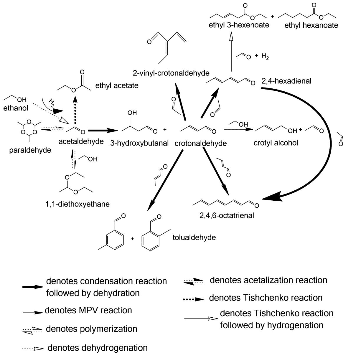
**Scheme 1.** Reaction network for acetaldehyde conversion over zeolite faujasite in liquid phase.
