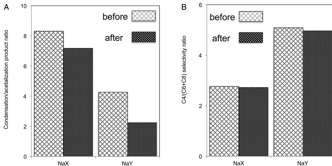
**Fig. 5.** Product ratios over NaX and NaY, before and after exposure to  $\text{CO}_2$ . (A) Condensation/acetalization ratio; (B) C4/(C6 + C8) condensation product ratio. The solvent (ethanol) to reactant (acetaldehyde) ratio was 10 by volume with acetaldehyde 2 mL. The reaction temperature was 230 °C and reaction time was 6 h. The catalyst weight was 400 mg.
