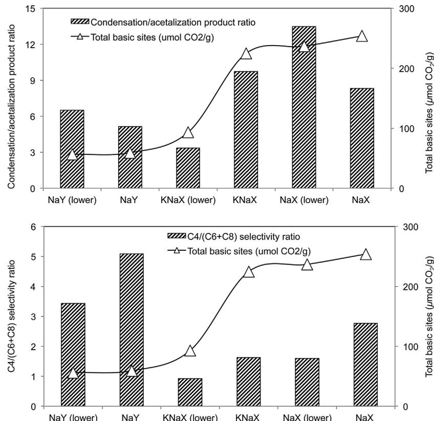
**Fig. 6.** Comparison among zeolites KNaX, NaX, NaY, and the corresponding not fully washed zeolites (lower-water). Reaction temperature 230 °C, reaction time 6 h, catalyst weight 400 mg, solvent (ethanol)/reactant (acetaldehyde) volume ratio 10, acetaldehyde 2 mL.
